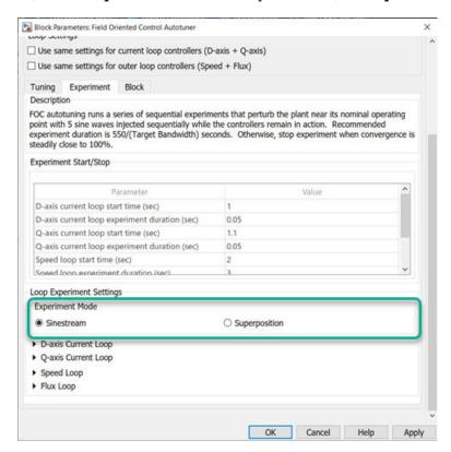
is useful when you have limited processing power and you want to reduce the execution time. To do so, on the **Experiment** tab of block parameters, set **Experiment Mode** to **Sinestream**.
